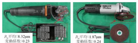
(a) Blaster tool (b) Disc grinding tool
