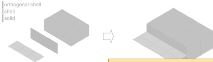
Fig. 1. The concepts of perpendicular shell-solid coupling. 出展 大沢ら Study on shell-solid coupling
