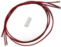
The connector is a Molex PicoBlade™ header, part number 53261-1071. It mates with Molex part number 51021-1000. Use crimp contacts 50058-8000 or 50079-8000.
